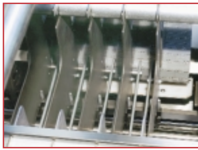
③ Servo-controlled grouper provides positive product handling and quick and easy changeover.
