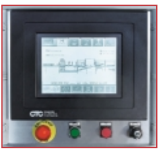
④ Graphic display, touch screen operator interface simplifies operation and provides checklist for changeover functions.
