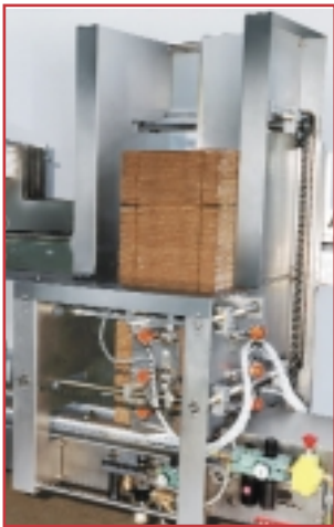
① Easy, continuous loading, vertical stack, high capacity blank magazine.
