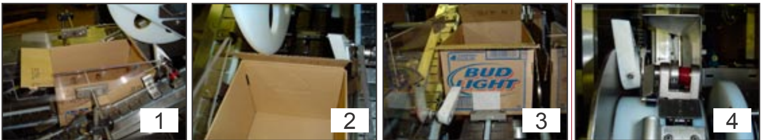
Figure 1.2 - Spring loaded tear-drop positioned to positively fold minor flaps.
