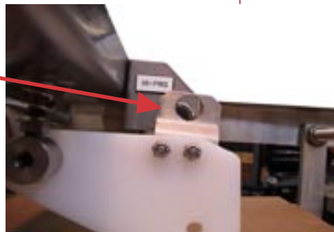
Figure 1.2 - Double blank causing detector to move upward and trip sensor
