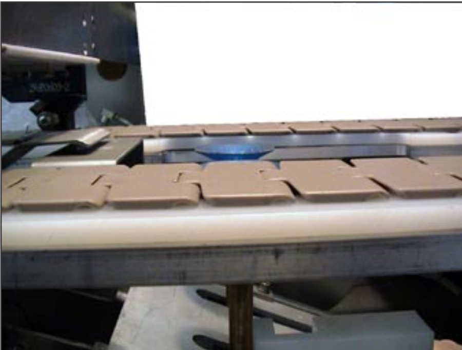
Figure 1.1 - Tray Magazine Vacuum Cups
