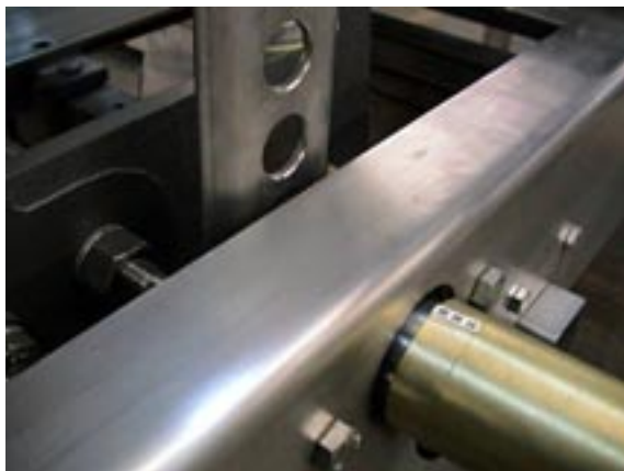
Figure 1.2 - Safety Solenoid and Slotted Plate
