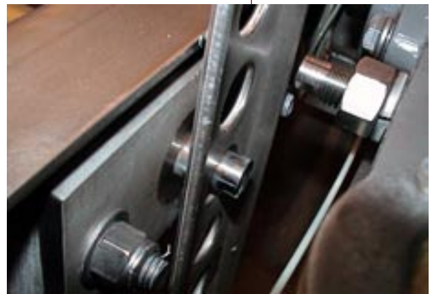
Figure 1.3 - Safety Solenoid engaged into Slot
